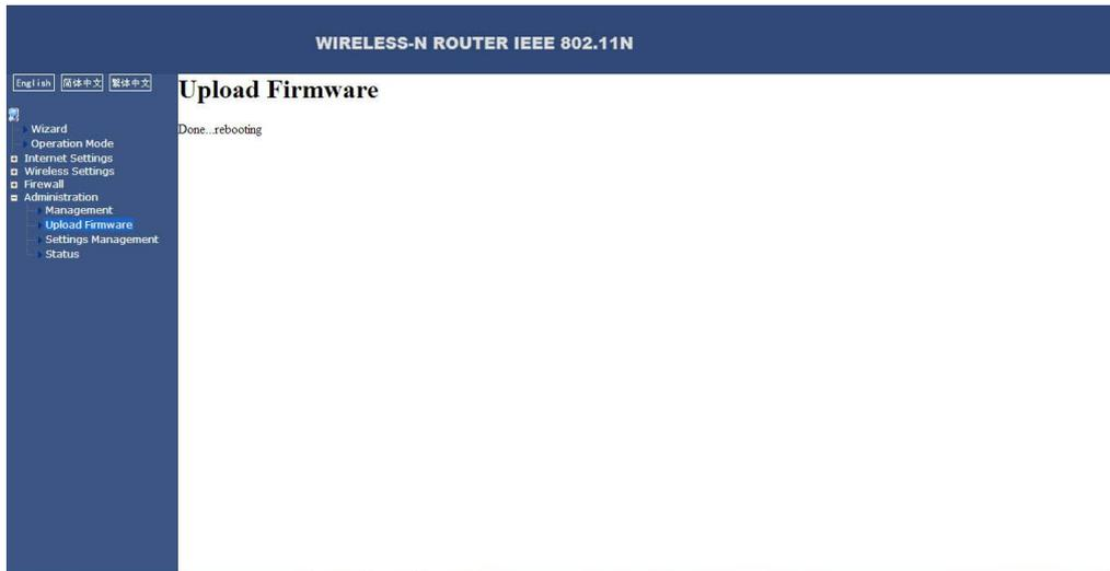
11. After upgrade please press RESET6 seconds to restart IX-T01 WiFi , after 1 minutes restart, we complete the firmware upgrade process.
